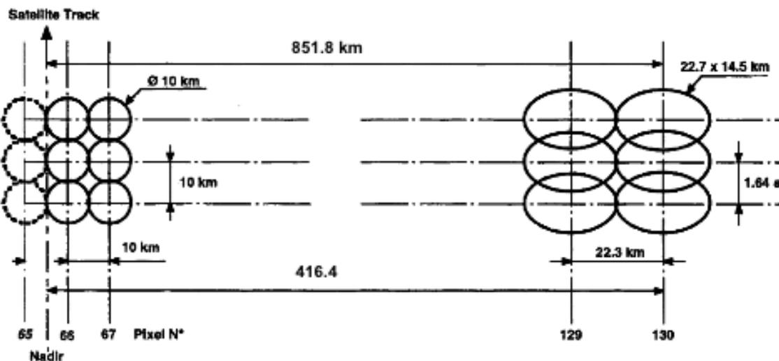
Figure 1: pixel representation on the ground for SAPHIR.
